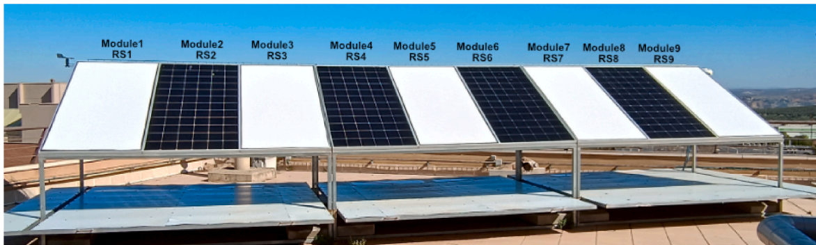
Fig. 4. Test bifacial PV system at the University of Jaén, Spain. Five of the nine PV modules were covered from the front to only absorb light from the back.
