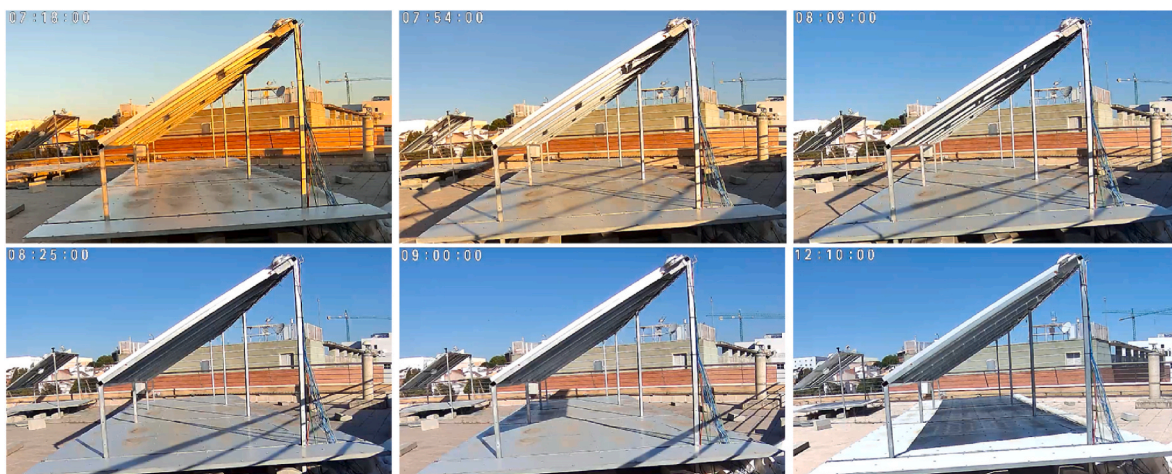
Fig. 3. Irradiance from the back side of a bifacial PV system in the morning hours of May 2024 in Jaén (37.79° N, -3.78° E). (Time is shown in CEST).
