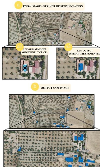
Fig. 6. Segmentation method to identify architectural elements in PNOA images. The input PNOA image (a) and the final segmented results (b).
