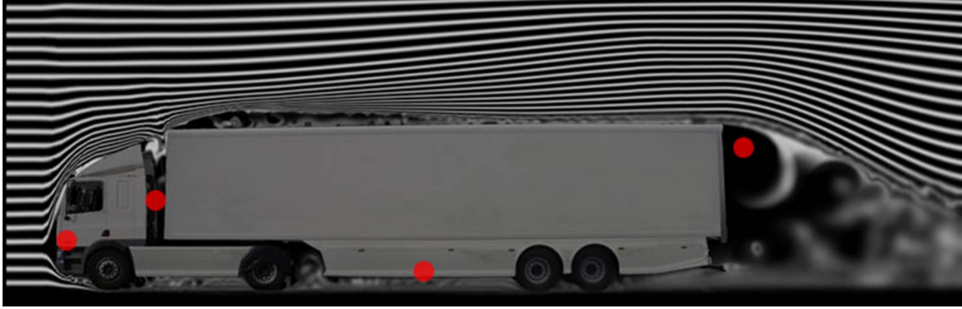
Figure 1.3: Four key locations for aerodynamics in a trailer truck [10].
