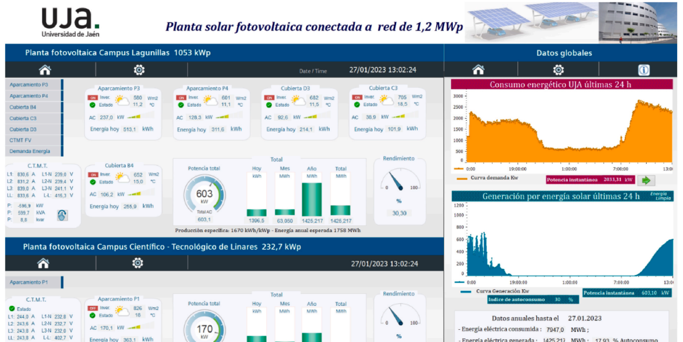
Fig. 7. Scada system used to monitor the UJA PV system.
