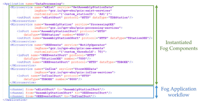
Fig. 10. XML document related to the application model of the DataProcessing Fog Application.
