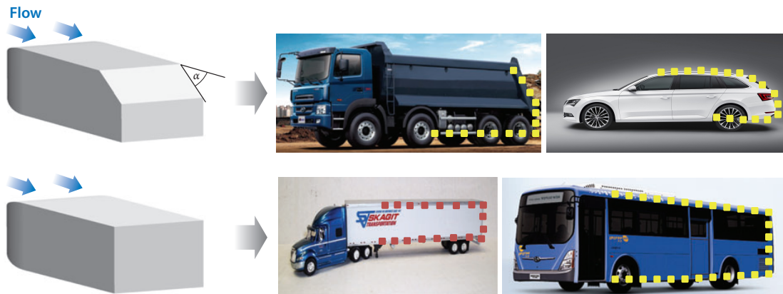
Figure 1.6: Simplified heavy vehicle models: slanted Ahmed body (top) and square-back Ahmed body (bottom), adapted from Choi et al. (2014).
