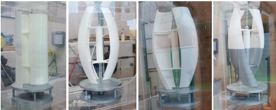
294 Fig. 7.- Rotors S and P j fixed to the wind tunnel by means of a circular PLA base.
