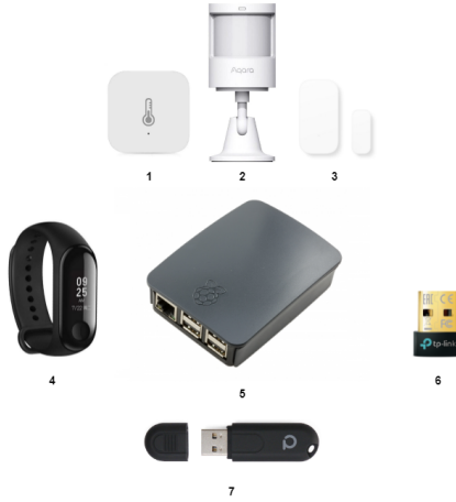
Fig. 1: Sensors and devices. 1 Temperature and humidity sensor. 2 Motion and light sensor. 3 Open and close sensor. 4 Activity tracker. 5 Nodes (Raspberry Pi). 6 Bluetooth adapter. 7 Conbee 2.
