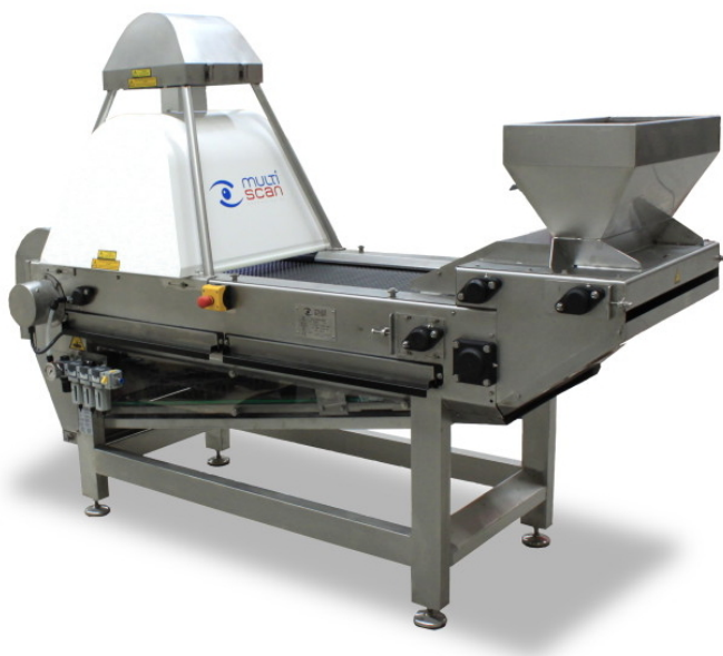
Figure 6.1 An example of commercial classification machine for table olives. Figure obtained from www.multiscan.eu .
