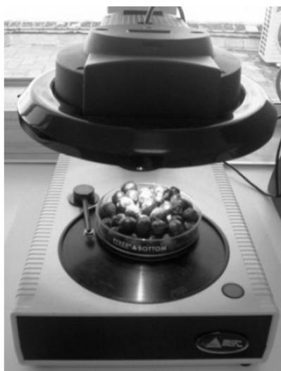
Figure 2.16 Sample turn table accessory of the spectrometer used in [38].
