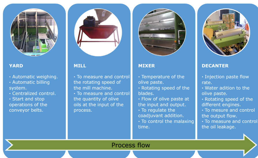
Figure 1.1 Possibilities for the automatic control of the virgin olive oil production process according to the different sub-processes of the production process; see Chapter 2 for more information.
