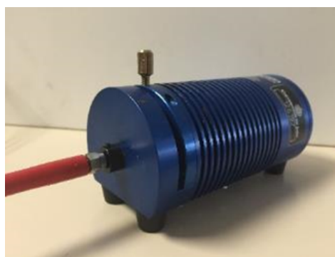
Figure 2.11 Halogen lamp housing, from which light is delivered through an optical fiber.
