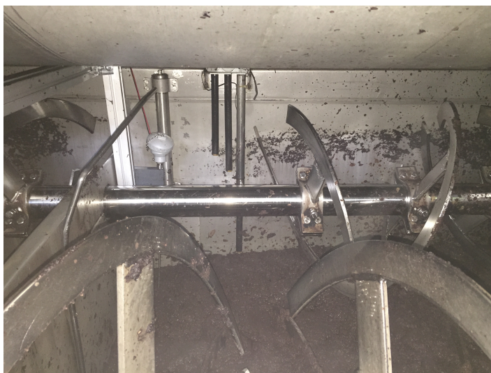
Figure 2.6 Picture of the inside of the thermomixer.
