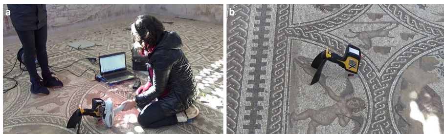
Fig. 3 In situ measurements using a both instruments (Bruker™ Tracer III SD® hXRF in white) and b the Olympus™ Innov-X Delta Premium hXRF with the soil foot (U8990900) accessory
