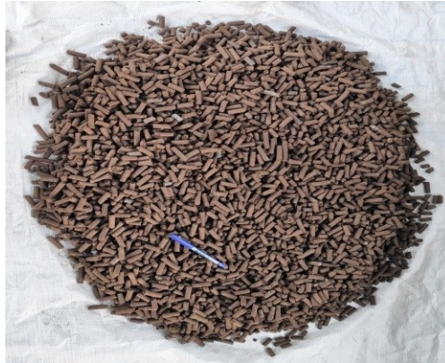
Figure 2: Exhausted olive pomace pellets used as feedstock to the downdraft gasifier.
