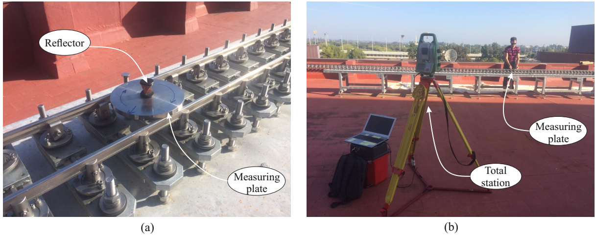
Figure 7: (a) Ellipsoidal measuring plate on the track. (b) Manual measurement of the track centre line
