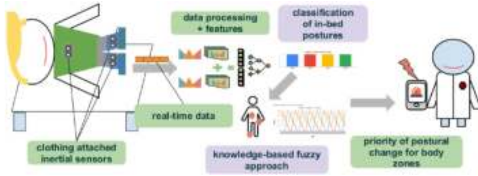
Fig. 1. Architecture of components: (i) inertial sensors attached to clothing, (ii) data-driven model for recognizing in-bed postures, (iii) knowledge-based fuzzy approach to compute the priority of postural changes for body zones, and (iv) a configurable threshold for notifications to caregivers.
