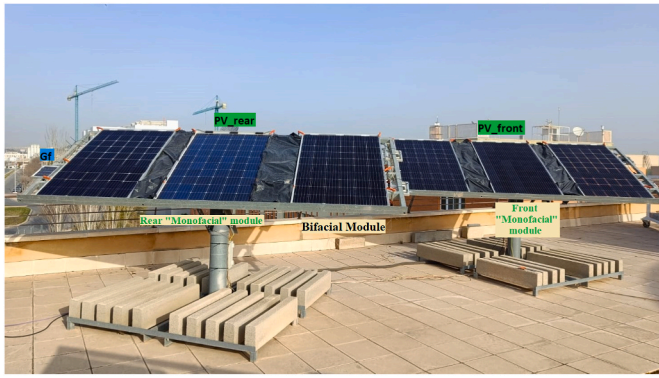
Fig. 1. Experimental set-up for the outdoors evaluation of the bifacial coefficient.
