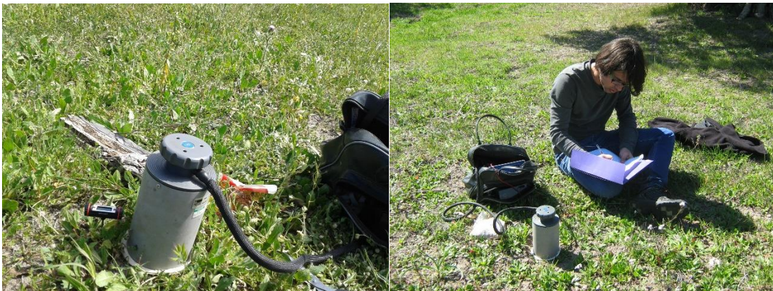
Figure 5. Images of the soil respiration measurements with PPSystem in Castillo de Canena property (Jaén).
