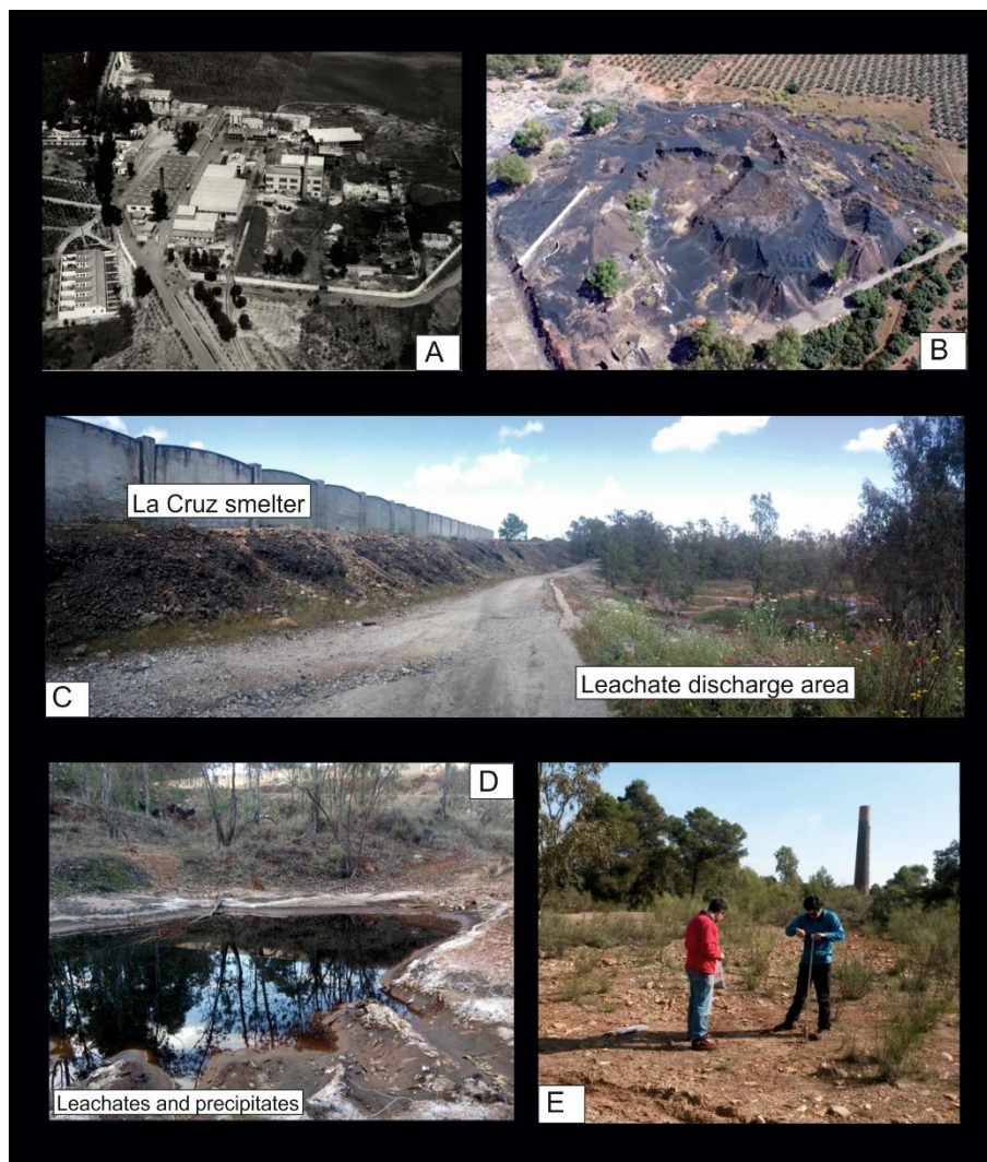
Figure 43. Pictures from the study area. a) Archive photograph showing the La Cruz smelter. b) Recent aerial view of La Cruz smelting slag. c) Wall surrounding the smelter facilities and leachates discharge at the foot of the slags. d) Leachates flowing from the facility drainage and precipitates generated by their evaporation. e) Sampling soils with an Auger tool. The big smelter chimney can be seen in the background.
