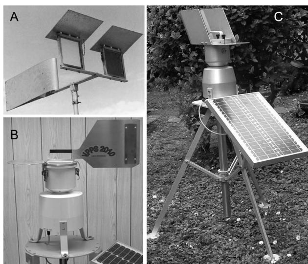
Fig. 1 Pollen samplers used in these aerobiological studies. (A) Cour pollen trap; (B and C) volumetric pollen traps based on the Hirst model, monitoring a known air volume per minute.
