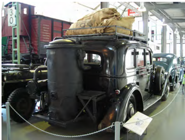
(a) German automobile fitted with Imbert-type wood gas generator in 1941 due to shortage of petrol. The wood gas drives a 6-cylinder four-stroke engine in series (power output: ~26 kW (36 hp); max. speed: ~70 km/h). On display at the Deutsches Museum in Munich, Germany. SOURCE: Mattes 1 .
