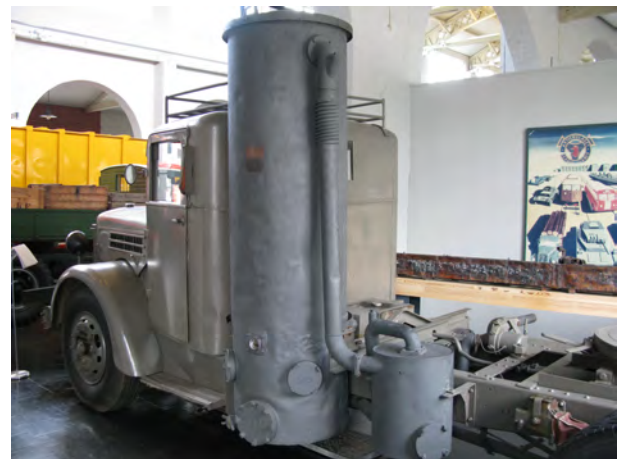
(b) Swedish truck from 1941 equipped with a wood gas generator. On display at the Scania Museum in Södertälje, Sweden. SOURCE: Herranderssvensson 2 .
