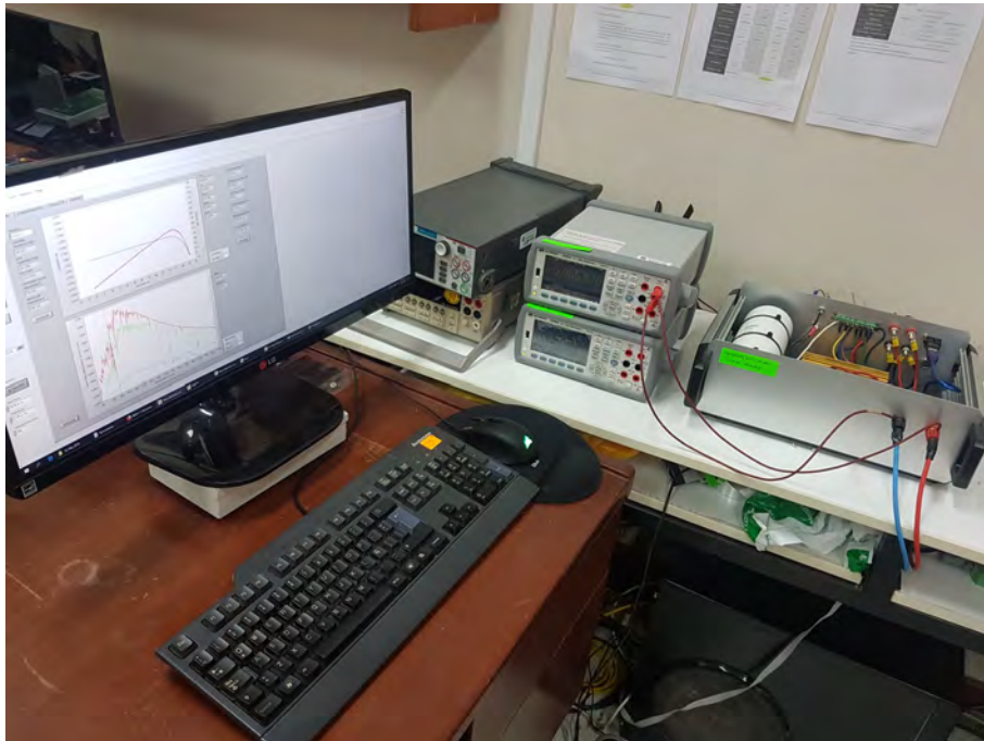
Figure 2.3: I-V tracer system.
