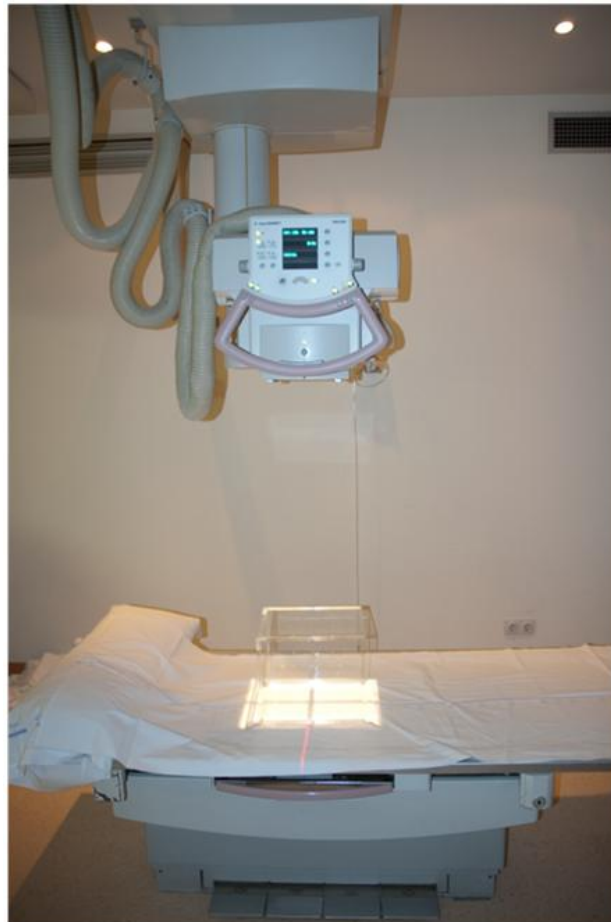
Figure 5. Prototype of locator object and X-ray system
