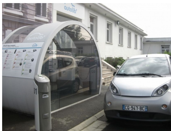
Figure 10. Parking space with a registration kiosk, a charging station and a Bluecar [48].
