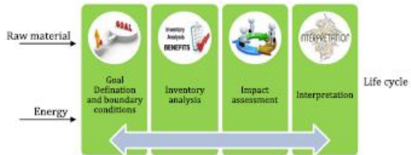
Fig. 4. LCA process as per ISO 14040 and ISO 14044 series standards.
