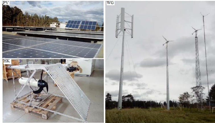
Figure. 5 Renewable energy sources available in the NG laboratory
