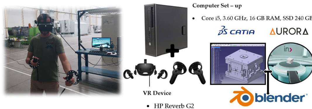
Figure 3. CAD—VR devices and environment.
