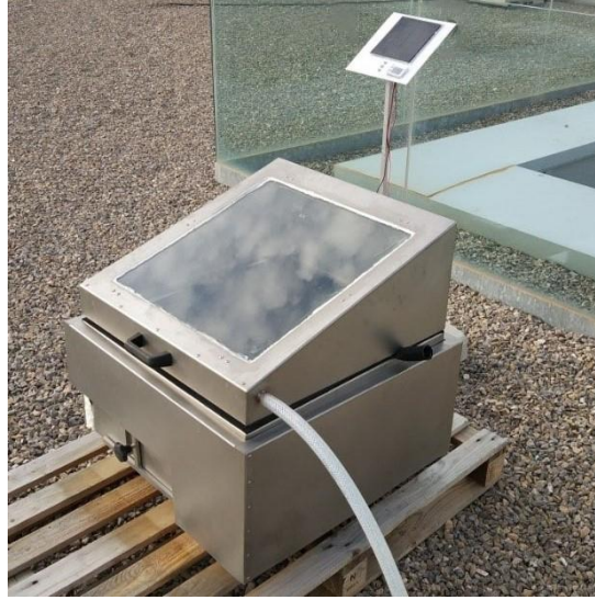
Figure 2. Photographic image of the solar still prototype.
