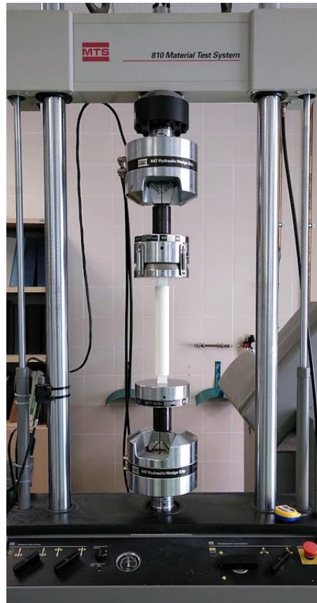
Fig. 10.- Uniaxial compression test of the mechanical element under study.
