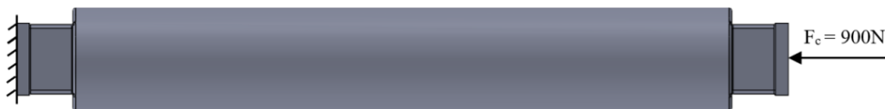
Fig. 3.- Boundary conditions and definition of the loads borne by the mechanical element.
