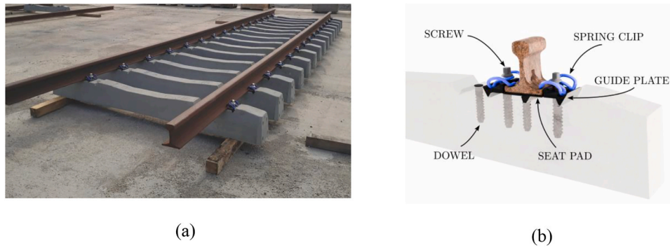
Fig. 2. Set up of rails and MMPC sleepers for the Iberian gauge (a) by using the SKL fastening system (b).
