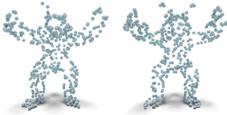
Figure 11: Sampling of the Armadillo mesh using the mt19937 pseudo-random sampler (left) and Halton sampling (right). On the left point cloud, the right ear of the model is missing.
