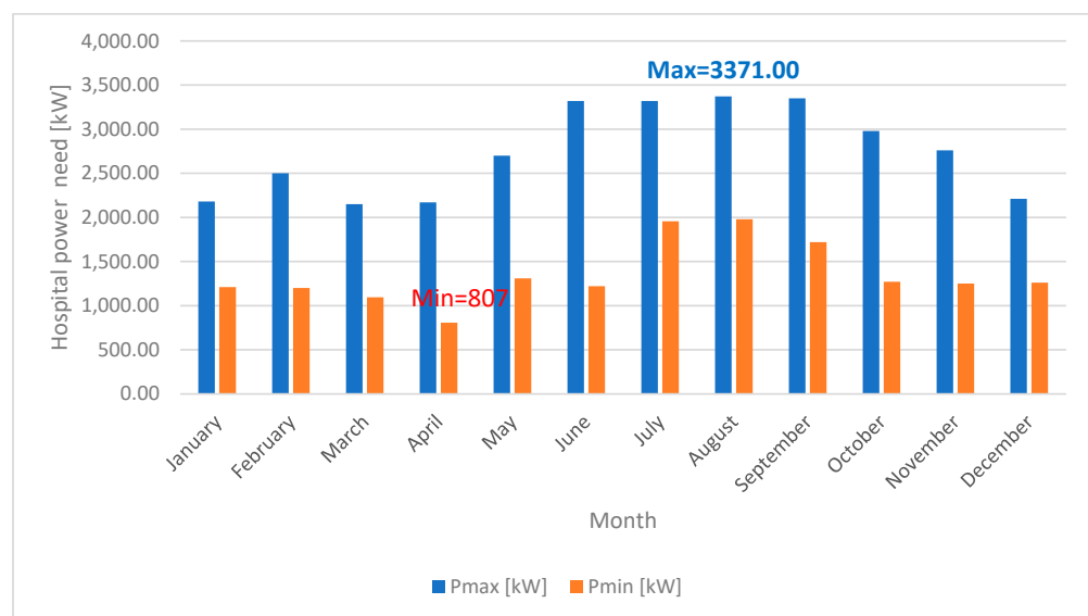
Figure 4. Historical time-series data for 2022 showing the hospital's electricity demand profile. The plot also highlights the minimum and maximum power demand recorded during the year: a minimum of 807 kW (on April 30th at 9:00 p.m.) and a maximum of 3371 kW (on August 10th at 2:00 p.m.).
