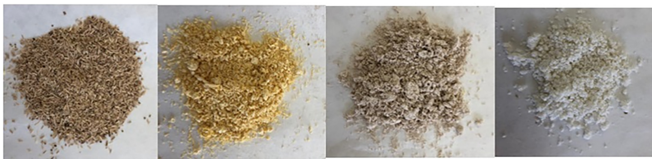
Figure 1. Visual appearance of OTP fibers. From left to right: raw OTP, OTP-AH, OTP-BH, and OTP-BL.
