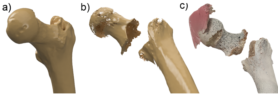
Figure 5.9: Image a represents the render of a femur before the experiment, b the render of the fractured femur and c the fractured bone obtained after the experiment.
