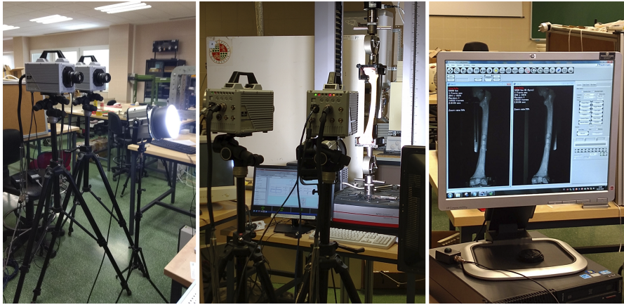
Figure 5.8: Camera system designed to capture the displacements resulting from the load applied to the human bone.
