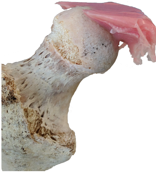
Figure 5.6: Proximal end segment of a femur with solidified resin in the femoral head.
