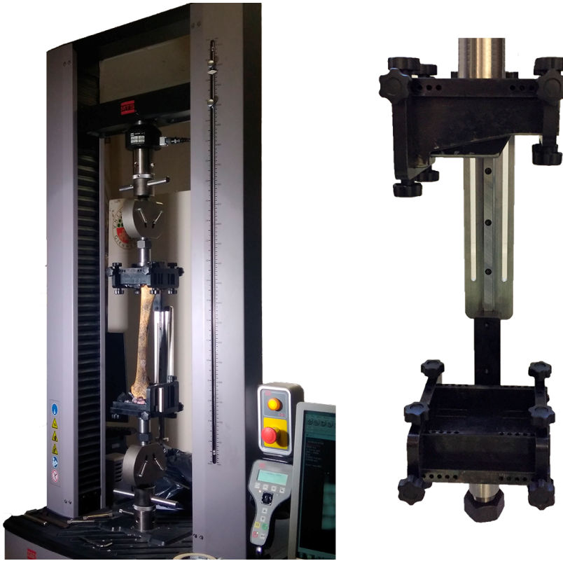
Figure 5.5: Universal machine for testing materials used with the fixture in which the bone is placed in the experiment.
