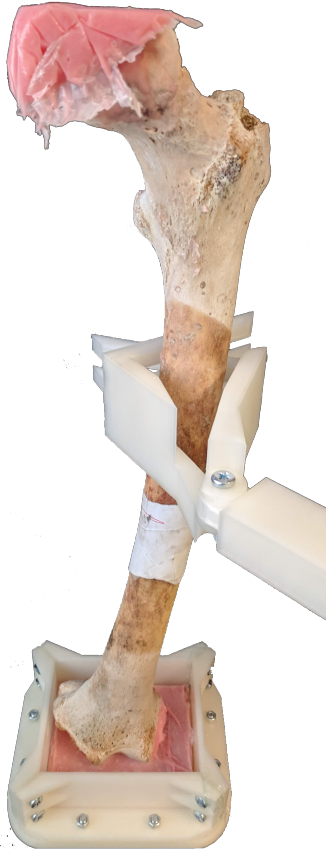
Figure 5.7: Femur placed on the 3D printing tool held by the clamp and resin in the areas that connect with the hip and knee.
