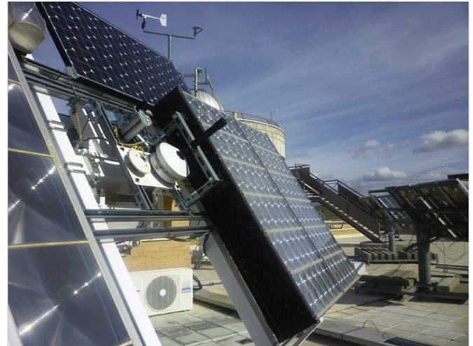
Fig. 1. Experimental setup for DNI and GI tracker option.
