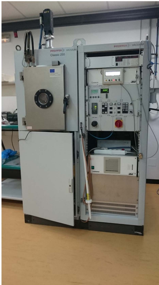
Fig. 2. In this figure appears the high vacuum evaporating chamber (Pfeiffer).
