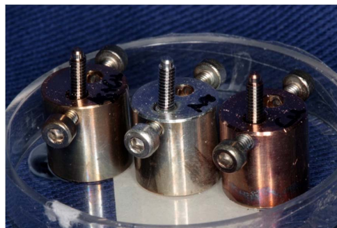
Fig. 3. Screws coatings. Ag-Cu (left), Ag (centre) and Cu (right).
