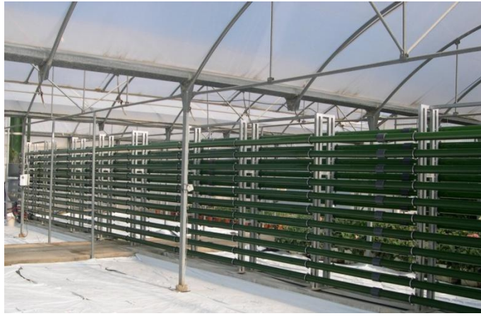
Fig. 1. Tubular photobioreactor ( 3 \text{ m}^3 ) at Estación Experimental Fundación Cajamar (EEFC) located in Almería, Spain.
