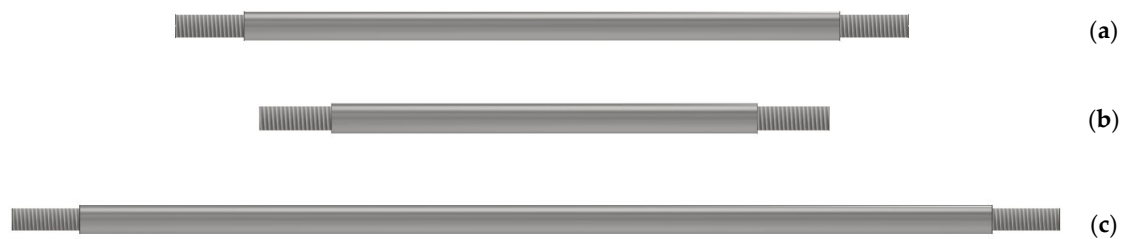
Figure 35. Three types of rod designed through extrusion: (a,b) related to steam exhaust and (c) related to steam intake.
