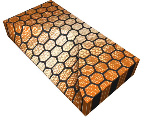
Figure 14: Example of complex composite. This composite is made of a core phase with honeycomb architecture and a matrix phase which is in turn a composite with fiber architecture and with higher core phase density at the endings. The microarchitecture is 2D as described in Section 4.5. The feature points for the honeycomb are located at the coordinates \{(0, 0), (1/2, 0), (1, 0), (1/4, 1/2), (3/4, 1/2), (0, 1), (1/2, 1), (1, 1)\} and periodic in \mathbf{u} and \mathbf{v} , with f_{core}(\mathbf{u}) = F2 - F1 . The fiber architecture was created with the feature point set \{(0, 0), (1, 0), (0, 1), (1, 1), (1/14, 8/16), (2/14, 4/16), (3/14, 12/16), (4/14, 2/16), (5/14, 10/16), (6/14, 6/16), (7/14, 14/16), (8/14, 1/16), (9/14, 9/16), (10/14, 5/16), (11/14, 13/16), (12/14, 3/16), (13/14, 11/16)\} , and f_{core}(\mathbf{u}) = F2 - F1
