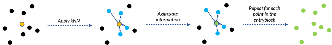
Figure 4: Dynamic graph building using kNN in EdgeConv.
