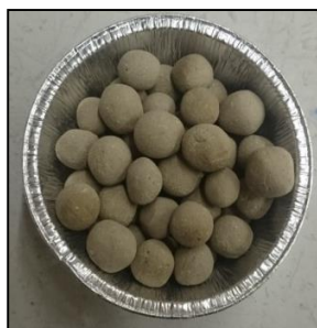
Image D.3.2.1. WBBS 15 samples after the sintering process.
