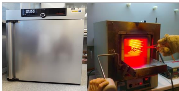
Image D.3.1.1. Stove (left) and muffle furnace (right).
