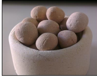
Image D.3.2.2. LWA s after sintering process (silico-aluminate container).
