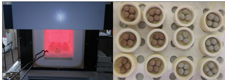
Image D.3.2.3. Furnace during sintering process and LWA sAP .
