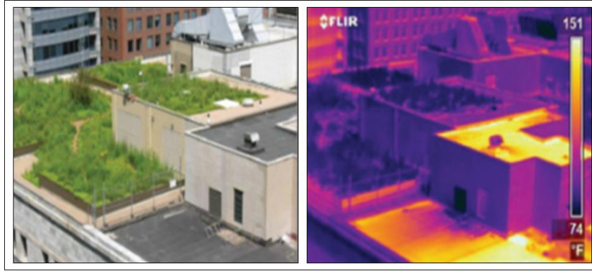
Image A.7.3.1. Thermal imaging. Green roof insulation capacity.
