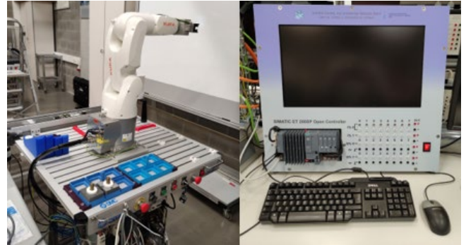
Fig. 2 Detail of the assembly cell: a) KUKA KR 3 R540 b) Siemens SIMATIC ET 200SP Open Controller.
