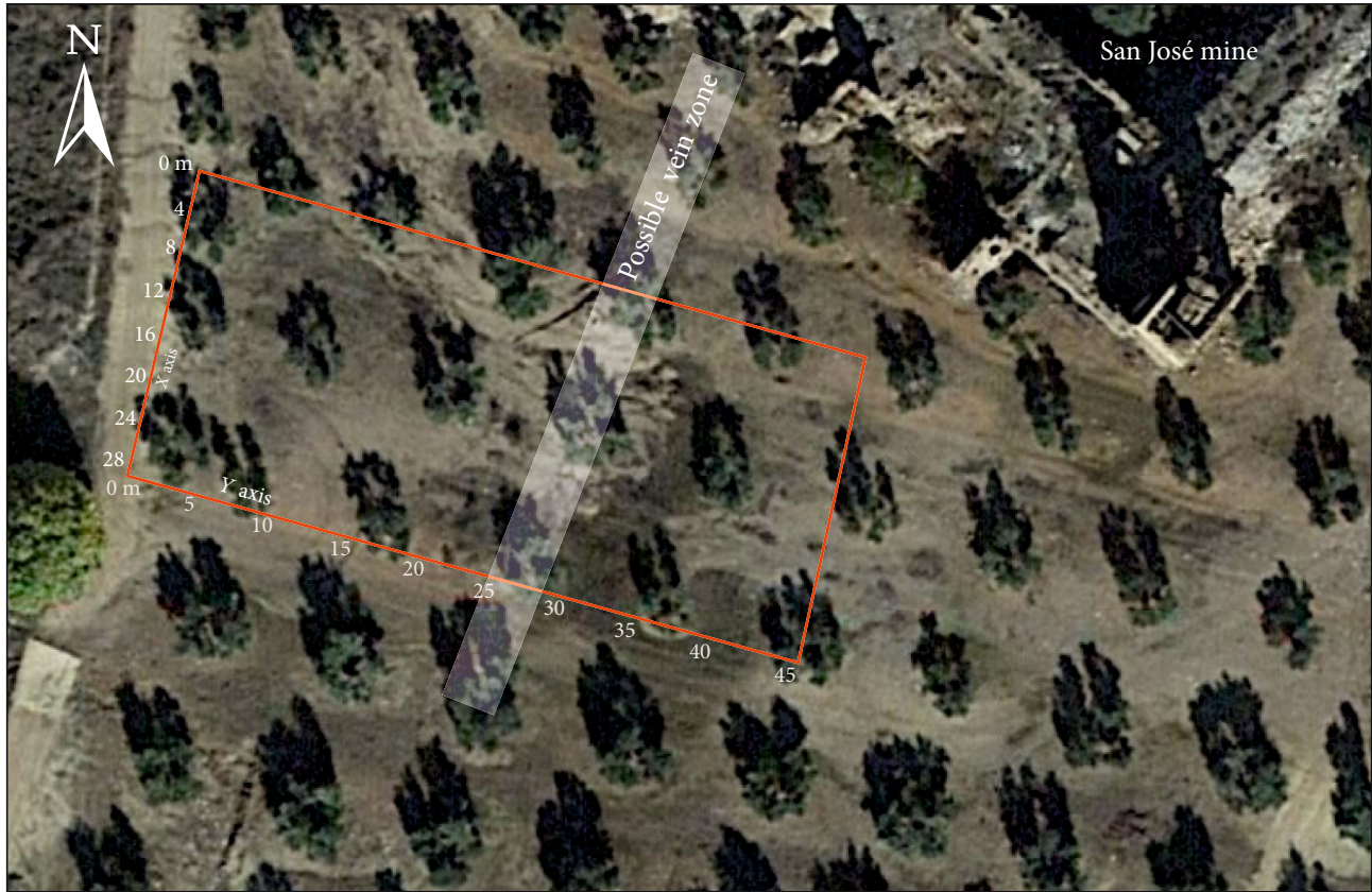
FIGURE 2: Aerial photograph showing the position of the studied grid next to the San José mine, in the Arrayanes mining concession. The supposed position of the vein trace is also marked.
