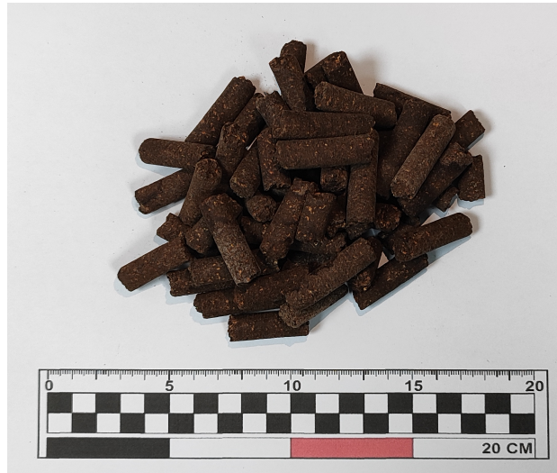
Figure 1: A sample of exhausted olive pomace pellets used as feedstock for the gasification plant.
