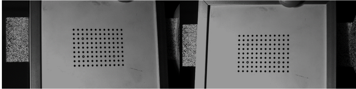
Fig. 25. Calibration grid from the point of view of the stereo-vision system for 3D-DIC measuring.
