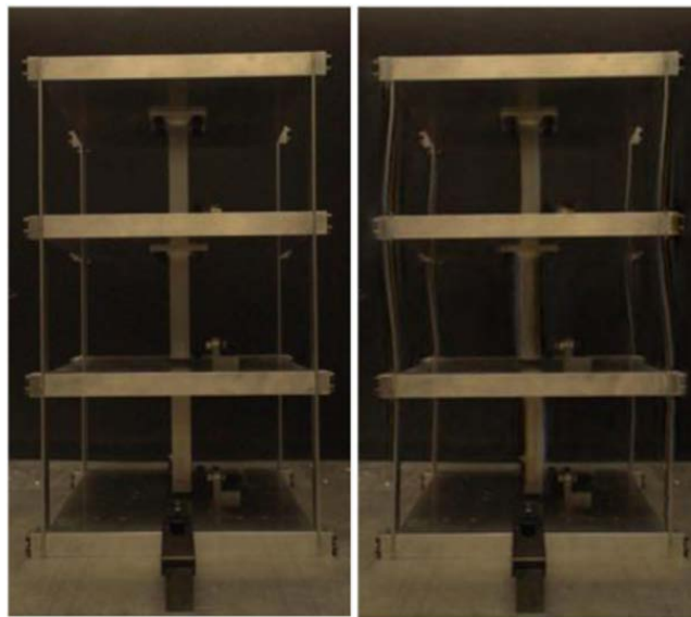
Fig. 17. Video stills of a three-story structure. (a) Non-magnified state. (b) Third mode magnified (Y. Yang, Dorn, Mancini, Talken, Kenyon, et al. 2017).
