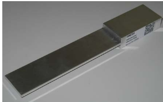
Fig. 19. Cantilever beam, employed for validation purposes of the methodology.
