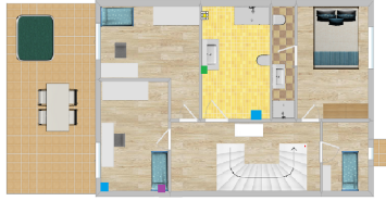
Fig. 4: First floor plan of the single-family house with the distribution of the devices.
