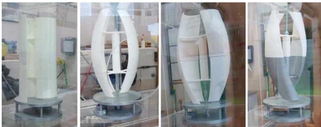
Fig. 7. Rotors \mathcal{R} and \mathcal{R}_j fixed to the wind tunnel by means of a circular PLA base.
