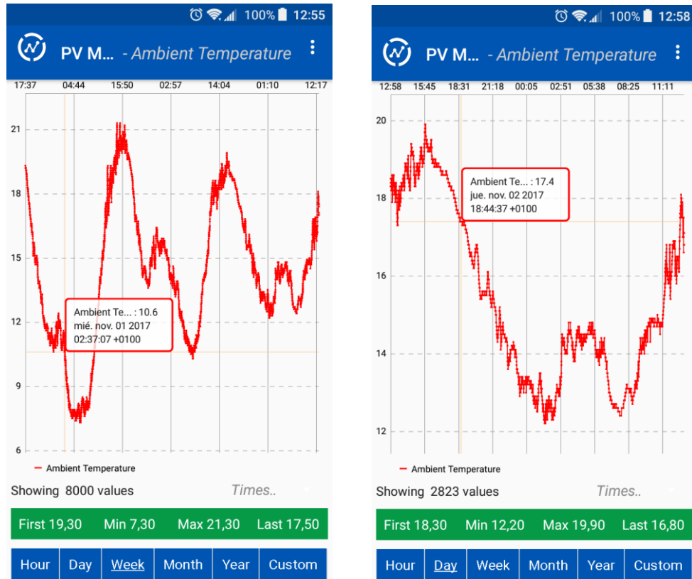
FIGURE 37: Screenshots on an Android smartphone using Thingview™ App: weekly (a) and daily (b) ambient temperature monitored by the datalogger located in Alcalá de Henares.
