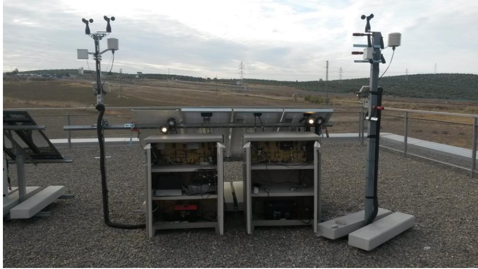
FIGURE 45: Two of the dataloggers installed in Linares: Datalogger SD version and Datalogger with a 3G connectivity version.
