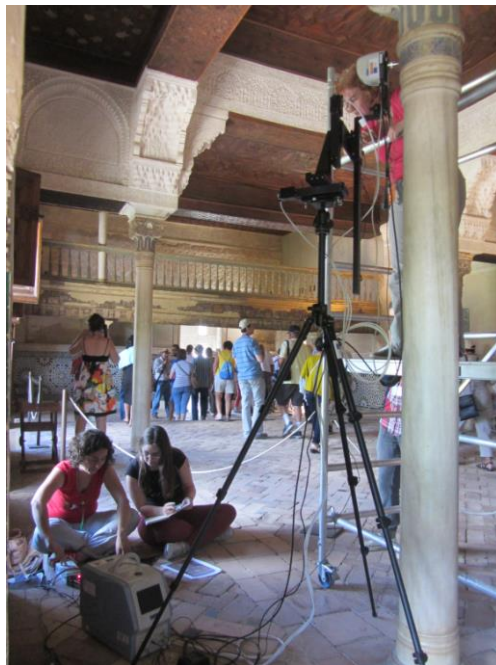
Figure 1. Portable Raman spectrometer working in situ in the Mexuar. Capital Mexuar B
