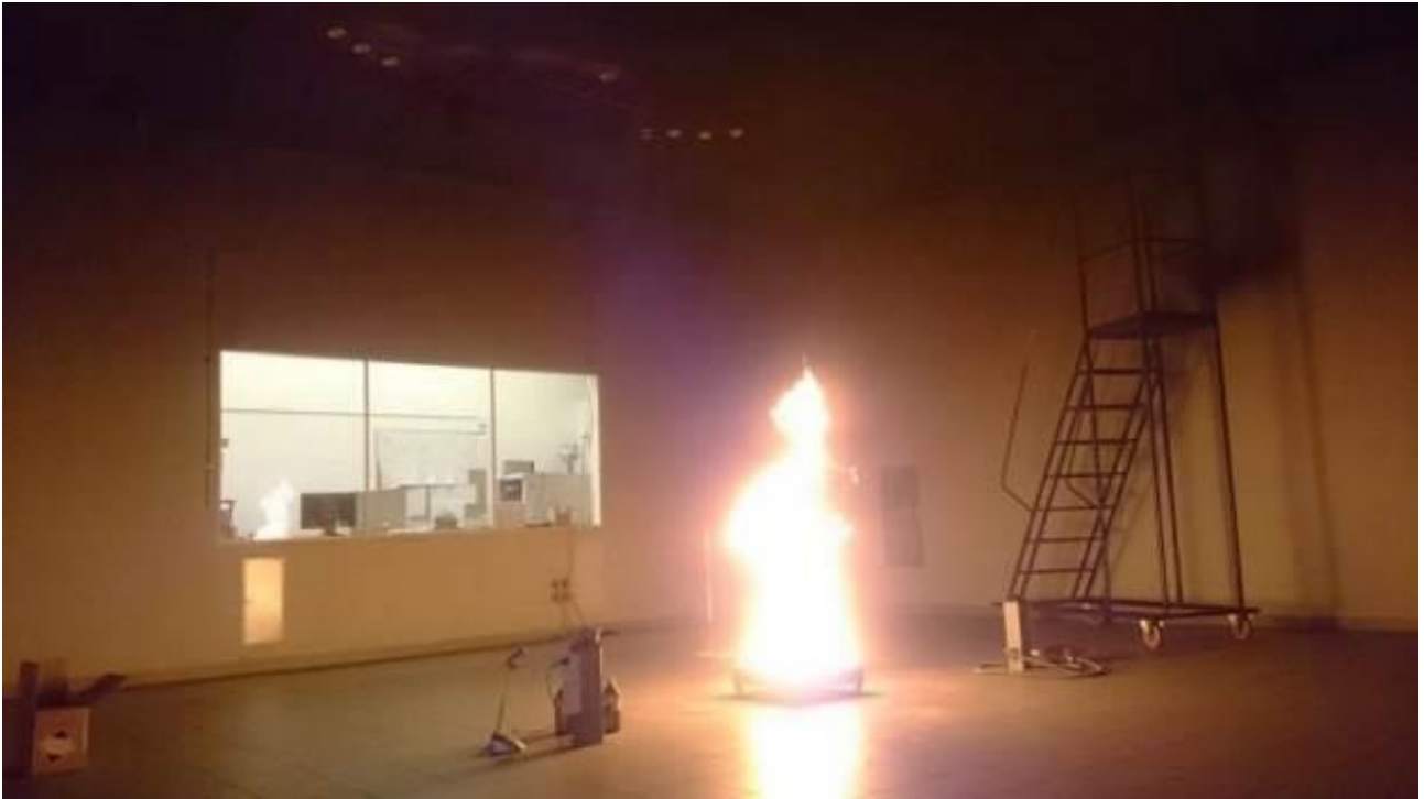
Figure 11 – ITB test chamber during each of the tests performed - Propanol, Y_s = 0.015 g/g
