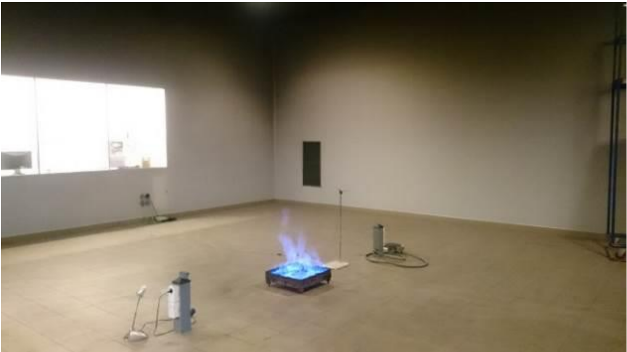
Figure 10 –ITB test chamber during each of the tests performed - Methanol, Y_s = 0.001 g/g
