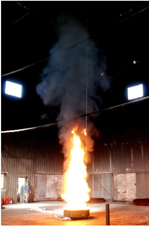
Figure 14 – Fire plume in one of the GX experiments (1a) and analytical representation of the fire plume (1b).
