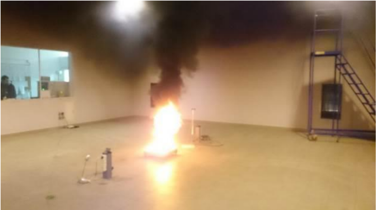
Figure 13 – ITB test chamber during each of the tests performed - Toluene, Y_s = 0.178 g/g.
