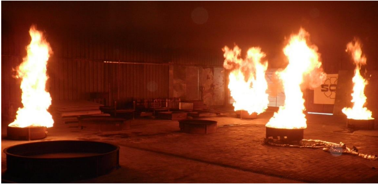
Figure 8 – Sequence of test #4FX showing the ignition of each pool fire (a-d) and when full regime is reached – i.e. all pool fire burning (e).
