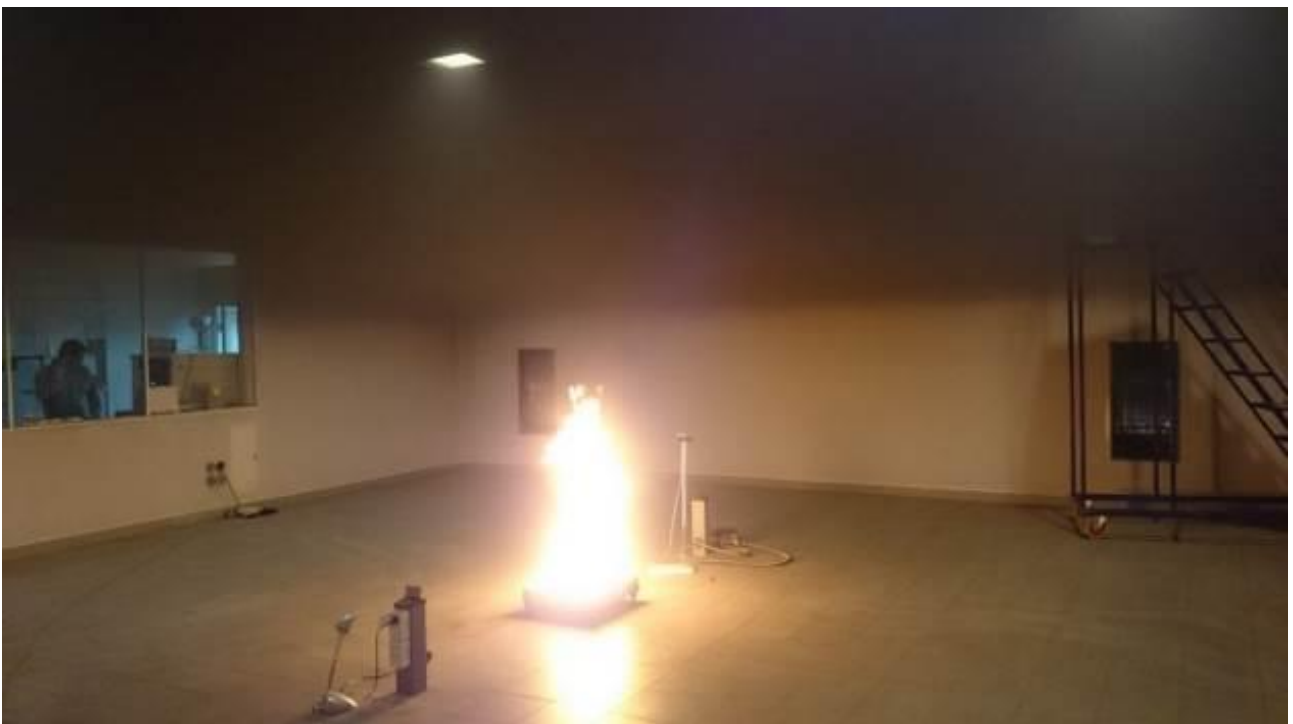
Figure 12 – ITB test chamber during each of the tests performed - Heptane, Y_s = 0.035 g/g
