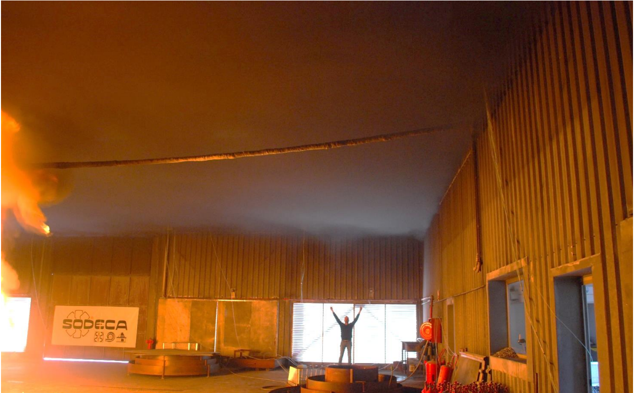
Figure 15 – Evidence of the smoke layer interface in one of the #GX tests.
