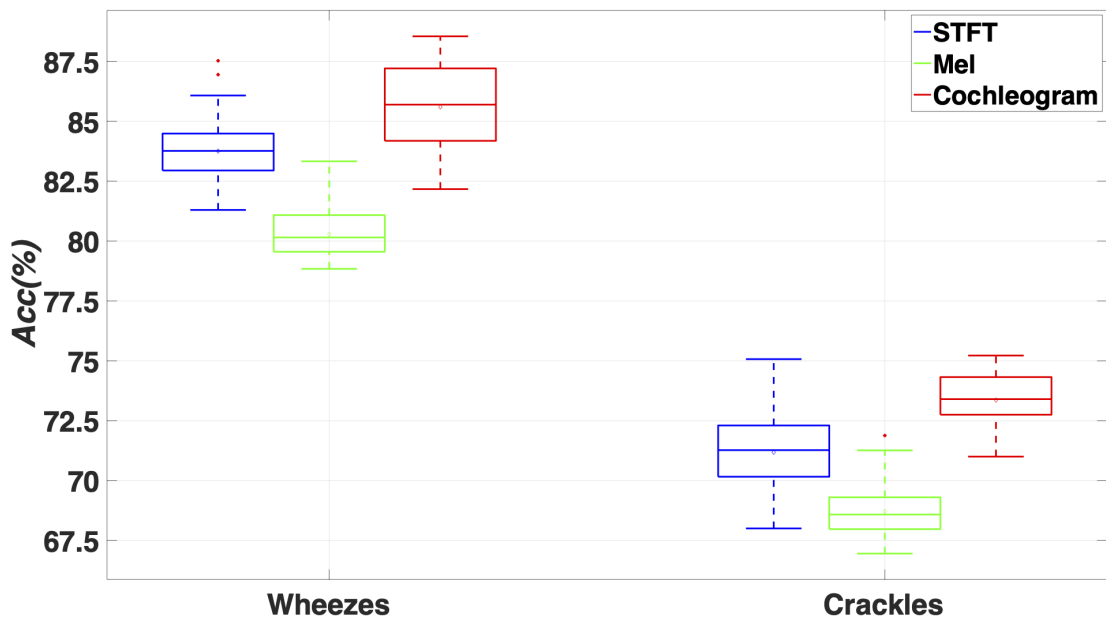
Fig. 5.2 Overall accuracy results evaluating the ICBHI dataset for the Cochleogram (window length of 8ms), STFT (window length of 32 ms) and Mel-scaled (window length of 32 ms) spectrograms using both the optimal values for the window lengths and overlap sizes. Each box represents 50 data points, each of them associated to a 10-fold cross-validation of the database evaluated. The lower and upper lines of each box show the first and third quartile. The line in the middle of each box represents the median value. The diamond shape in the center of each box represents the average value. The lines extending above and below each box show the extent of the rest of the samples, excluding outliers. Finally, outliers are defined as points that are over 1.5 times the interquartile range from the sample median, which are depicted as crosses.
