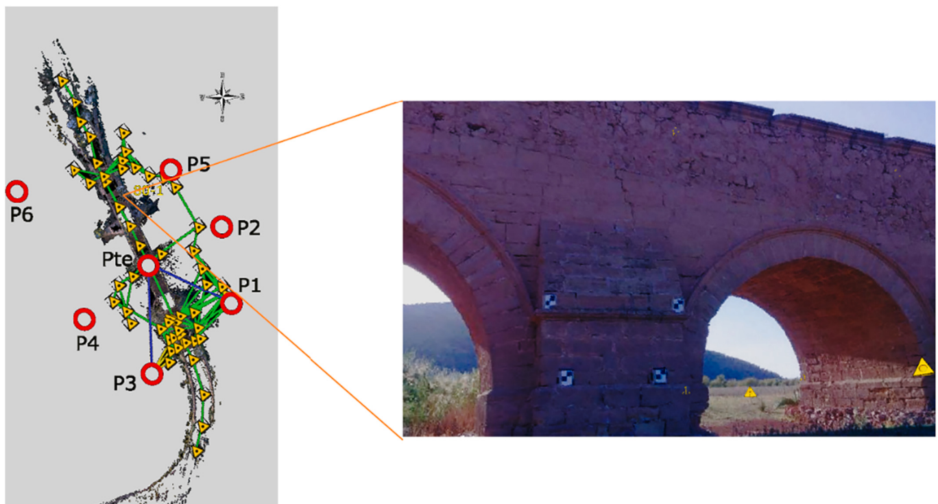
Fig. 6. Positional quality control from the registered survey using targets.
