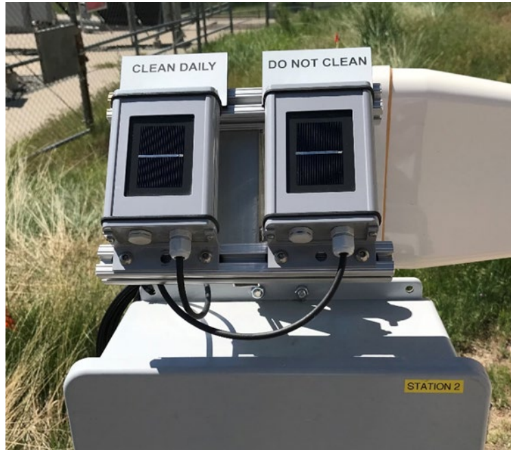
Figure 1. A typically manually cleaned soiling station with small silicon reference cells.
